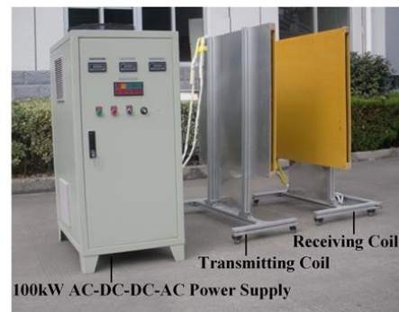
Fig. 8: Diagram of the wireless charging experiment device with 100 kW input power
